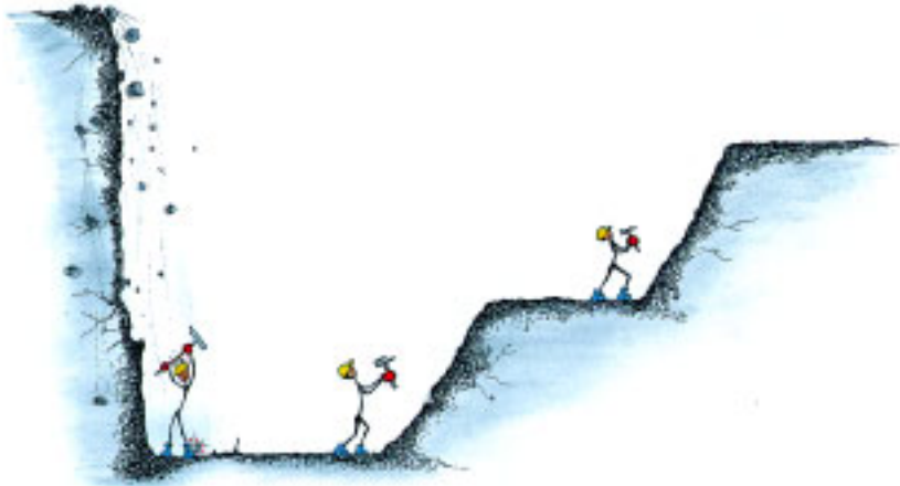
Unsafe steep pit wall.
